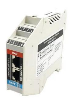
Ethernet LAN ports are marked as HAZ and SAFE. Network connections in explosive hazardous areas must be connected to the RJ45 connector marked HAZ, while downstream devices located in non-hazardous areas must be connected to the RJ45 connector marked SAFE. It is recommended to use an RJ45 Cat5e cable. LAN connections to explosive hazardous areas are marked with a blue color on the label to prevent confusion
